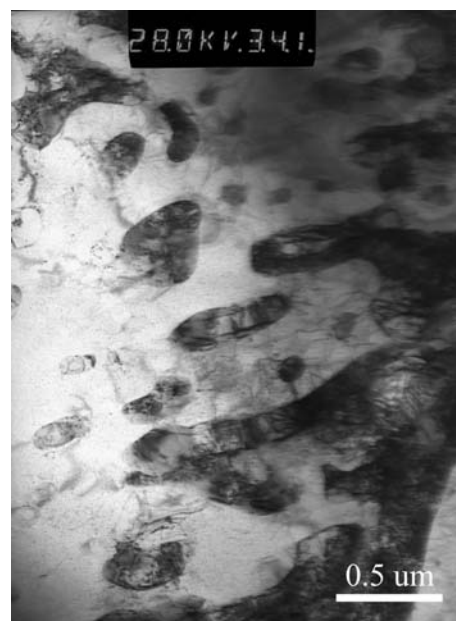
Fig. 11 Bright-field TEM image of granular nitrogen pearlite: no specific orientation relationship between the ferrite and the globulized nitride \gamma' -Fe 4 N
